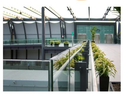
CANAL is often tasked with producing bespoke architectural metalwork incorporating glass on a large scale for commercial projects. Having previously produced bespoke architectural metalwork for BAA the reputation of CANAL secured the contract for the expansion of Gatwick's North Terminal; Supplying 500 metres of balustrade using 20mm thick mild steel balusters, laminated glass, all finished with satin polished hand and trolley rails.
